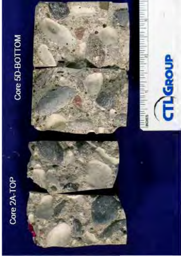
Fig. 7 Image showing freshly fractured surfaces of Cores 2A-TCP and 5D-BOTTOM. The fracture surfaces pass around almost all coarse aggregate particles indicating a weak paste-aggregate bond. Scale is marked in inches.
