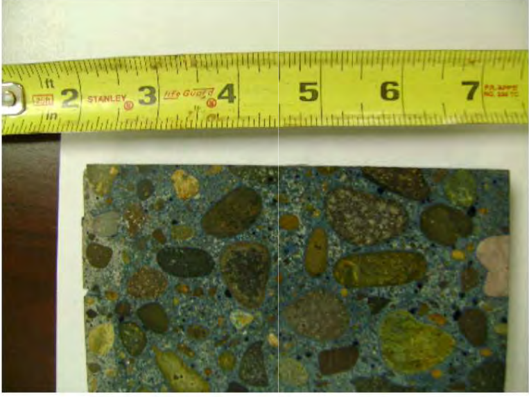
Photograph #2 - Sample 06033-2. Color change can be seen in paste at top surface as well as the bulk paste.
