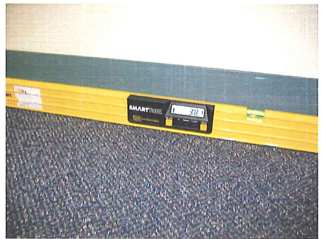
Sloping floors with up to 3/8" per 4 feet measured on the fifth floor
