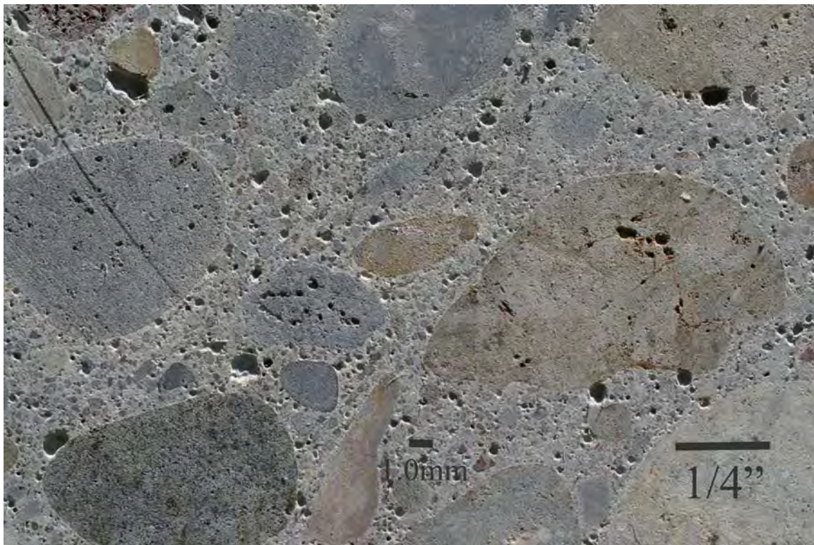
FIGURE 5 Sawed longitudinal surface shows typical appearance of aggregates and air-void system.
