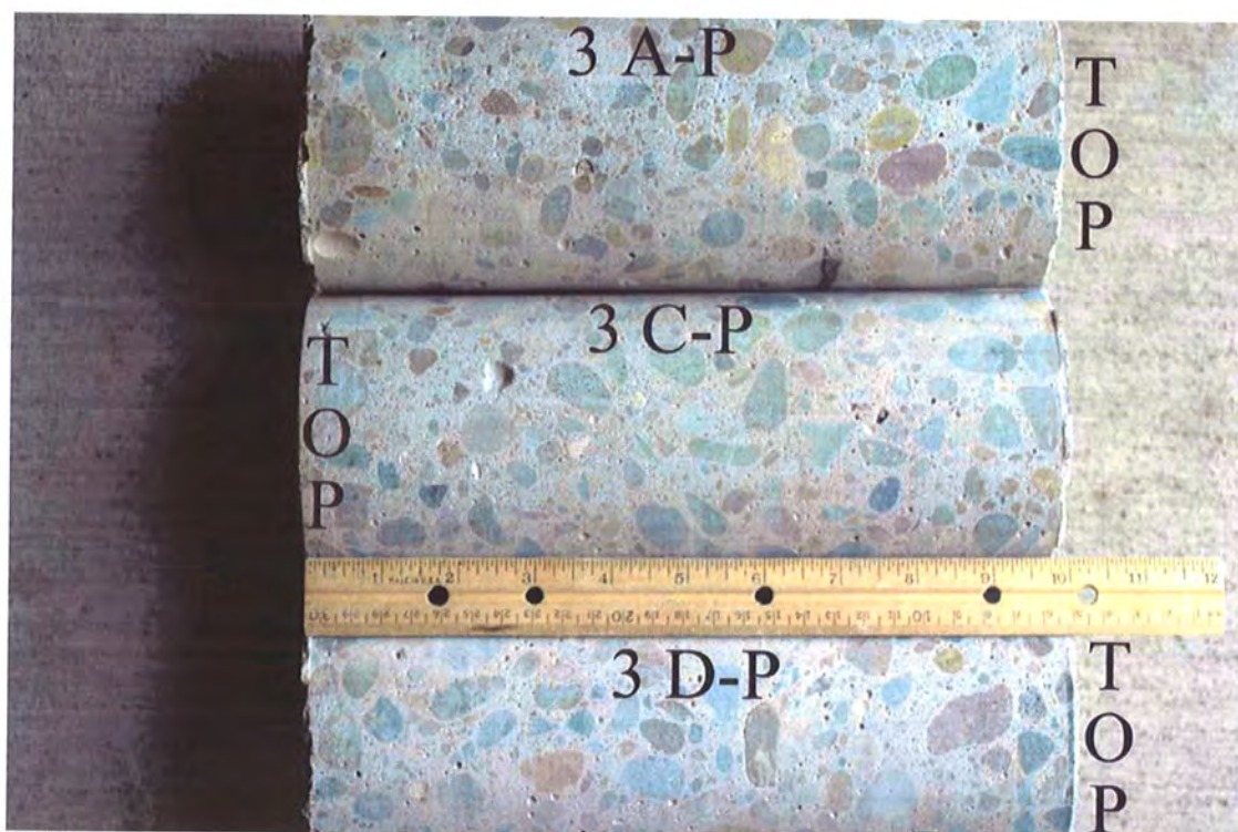
FIGURE 14 Side of 3-P Series cores as received shows aggregate size, shape and distribution and larger voids.
