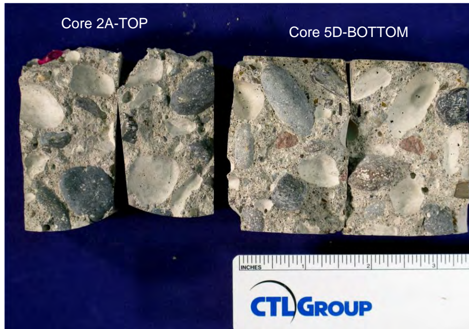
Fig. 7 Image showing freshly fractured surfaces of Cores 2A-TOP and 5D-BOTTOM. The fracture surfaces pass around almost all coarse aggregate particles indicating a weak paste-aggregate bond. Scale is marked in inches.
