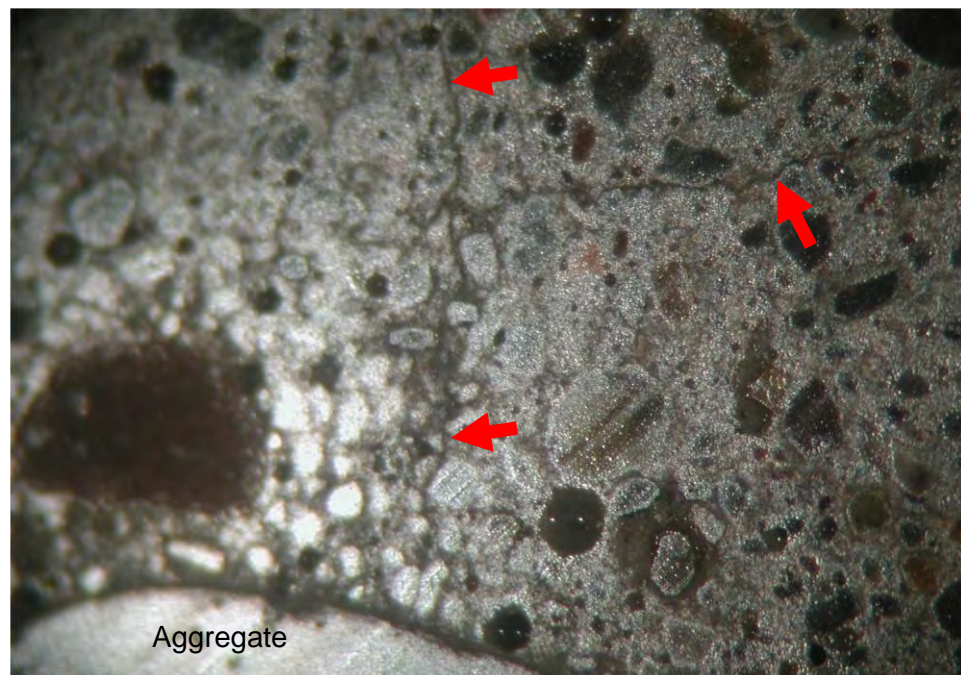
Fig. 10 Stereomicroscope image of a cut and lapped cross-sectional surface of Core 3C-MIDDLE, showing microcracks in the paste between coarse aggregate particles (arrows). The image was taken using oblique illumination shortly after the surface was wetted to highlight the microcracks. Field of view is approximately 0.5 in. across.
